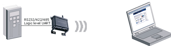
Picture 2. The Serial Port Adapter connected to the controller communicates wirelessly with a Bluetooth enabled Laptop.
